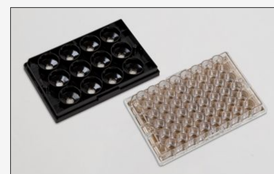
Multiwell MEAs: MEMS processes were developed to distribute 768 nano-textured microelectrodes (30 μm in diameter; 25 KQ @ 1KHz) across large-area, SBS-compliant plates
