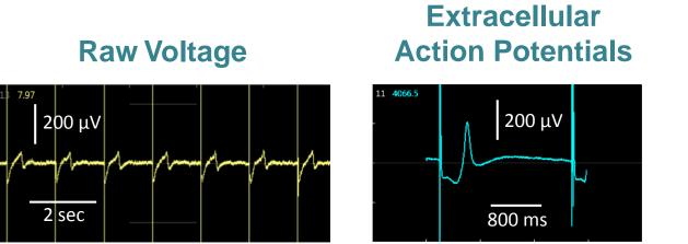
Raw voltage signals are processed in real-time to obtain extracellular field potentials from across the network, providing a valuable electrophysiological phenotype for applications in drug discovery, toxicological and safety
