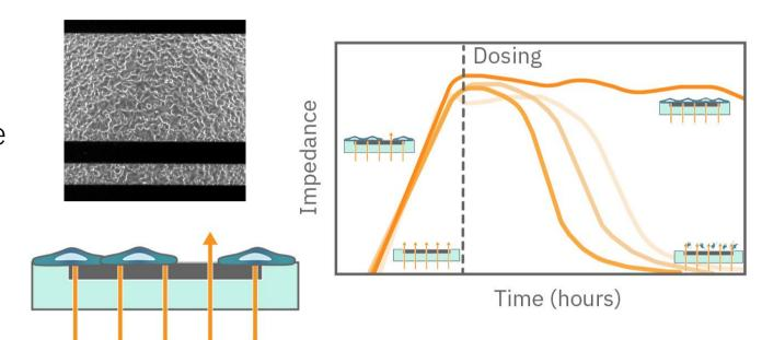
The impedance is measured from electrodes embedded in the bottom of each well. As cells cover more of the electrode, impedance increases in proportion to the number of viable cells. If a perturbation kills the attached cells, impedance decreases as the cells lyse.
