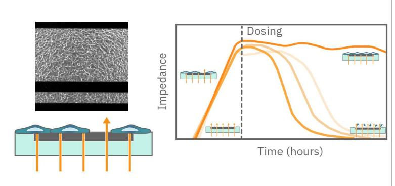
The impedance is measured from electrodes embedded in the bottom of each well. As cells cover more of the electrode, impedance increases in proportion to the number of viable cells. If a perturbation kills the attached cells, impedance decreases as the cells lyse.
