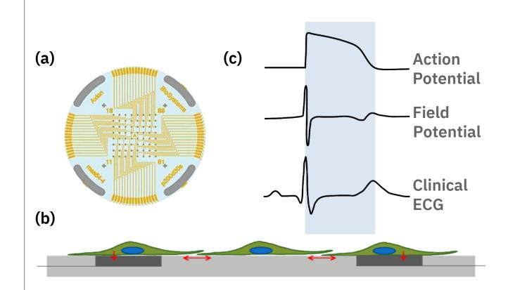
A planar grid of microelectrodes (a) interfaces with cultured neurons or cardiomyocytes (b) to model complex, human systems. Electrodes detect changes in raw voltage and record extracellular field potentials (c). The same microelectrodes can track cell viability using impedance measurements.
